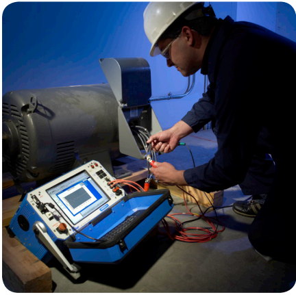
Testing a stock motor with a Baker AWA-IV for quality assurance before placement in service
